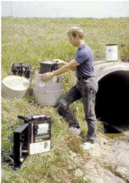
**An area velocity flowmeter, sampler, and rain gauge form a system for monitoring storm water runoff.**
