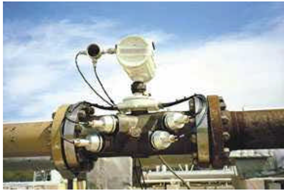
A Daniel ultrasonic natural gas flowmeter inline for calibrating at Southwest Research Institute.
