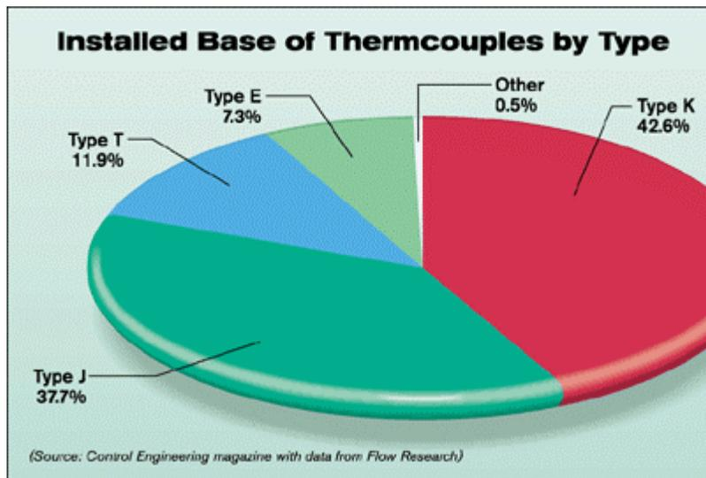
Broad applicability and inherent linearity have made Type K and J thermocouples the most used temperature sensors in industry.
