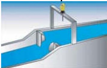
The most common instrument for non-contact open channel flow is an ultrasonic gauge, but pulse radar's microwave energy, unlike sound waves used in ultrasonic measurement, is not affected by steam, mist, or foam generated by the combination of heat and chemicals that exists in some industrial open-channel measurements. A pulse radar gauge can be programmed to output the flow for any type of flume or weir, making it as adaptable as any other technology on the market.
