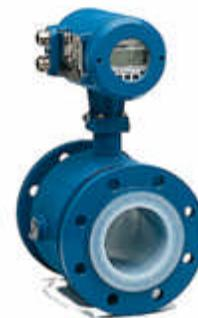
Magnetic flowmeters use wire coils mounted on or outside of a pipe. Current through these coils generates a magnetic field inside the pipe section. As conductive liquid passes through the pipe, it generates a voltage detected by electrodes mounted on either side of the pipe. The magnetic flowmeter uses this voltage to compute flowrate.
