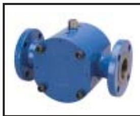
lobes. This lowers the pressure drop; creates no axial, side, or end loads; and allows the flowmeter to be used with high and low-viscosity liquids from light hydrocarbons to asphalt. Line sizes are 1-4 in., flow rates are up to 700 gpm, and viscosities are up to 10,000 cP.
