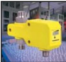
and gases. The solid-state sensors have no moving parts, connect directly into a pipeline with no intrusive probe, and are available with a discrete transistor output or 4-20 mA output. Setup uses adjustment pots on the front of the housing. All wetted parts are 316 stainless steel.
