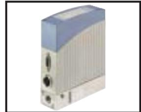
20 ml/min to 50 l/min. Accuracy is 1% of the reading and 0.5% FS, and linearity is 1% FS. Maximum inlet pressure is 145 psi, depending on valve diameter. Fieldbus communications include Profibus-DP and DeviceNet. The device can be calibrated on two different gases and switched between gases by the user.
