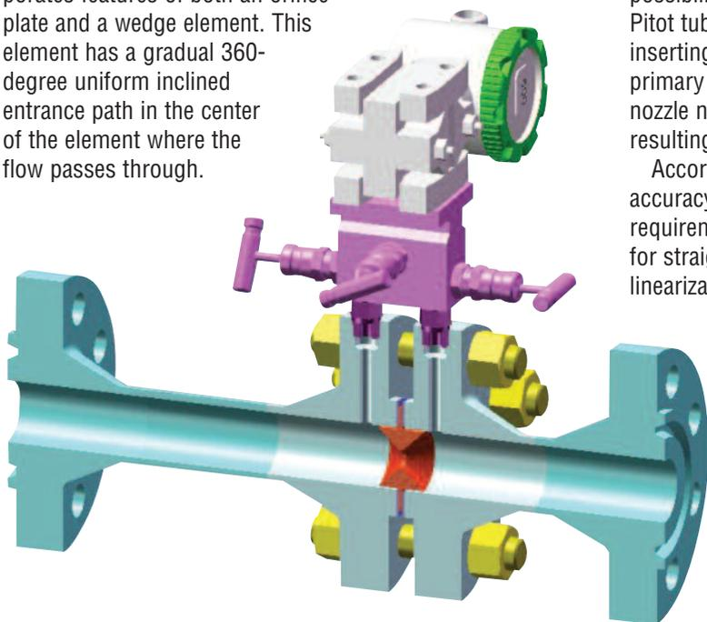
*Densipro's Torus Wedge design is a circumferential wedge element that incorporates features of both an orifice plate and a wedge element.*
