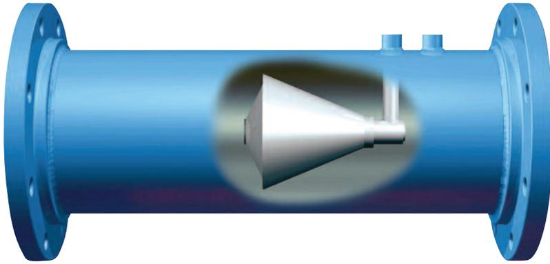
McCrometer's V-Cone primary element consists of a contoured cone suspended inside a straight pipe. As the flow passes the cone, short vortices are formed with a low amplitude and high frequency signal.
