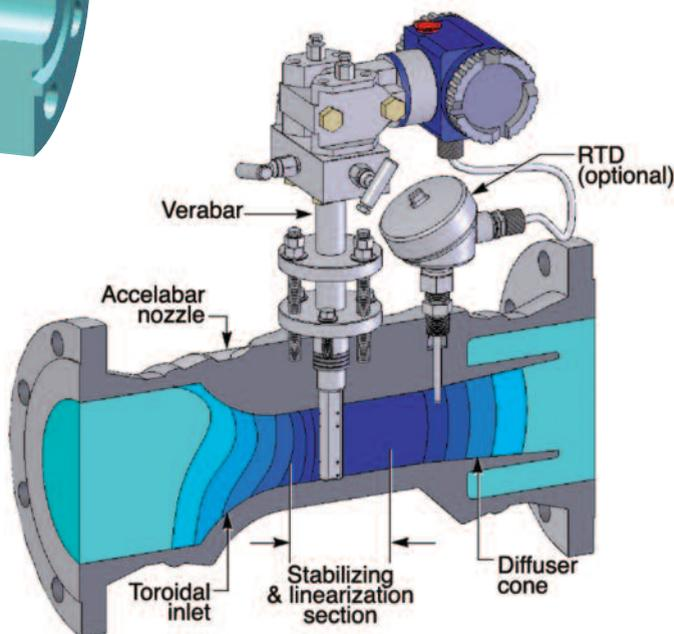
*Veris's Accelabar is a primary element that places an averaging Pitot tube inside a flow nozzle.*
