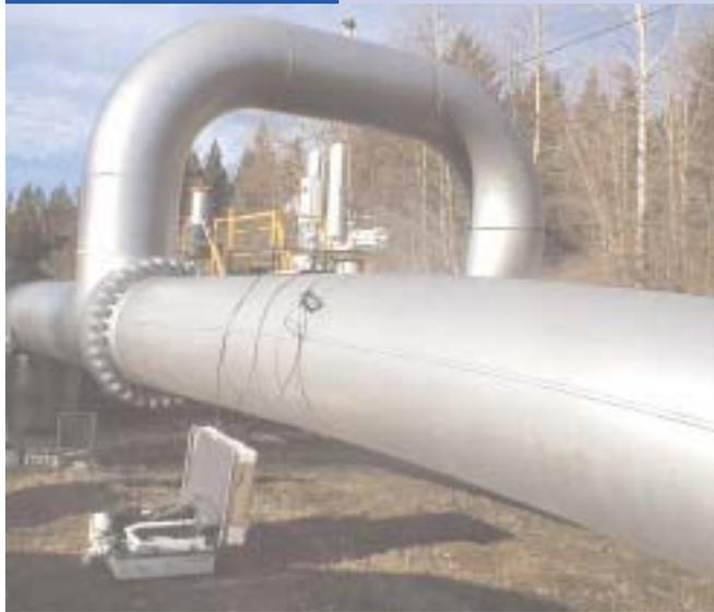
The GC868 ultrasonic flowmeter, a new clamp-on flowmeter from Panametrics, shown during a demonstration at West Coast Energy's main natural gas transit line coming into U.S. The application is 36-inch outer diameter, 0.5-inch wall thickness and pressure of 700 psig.
