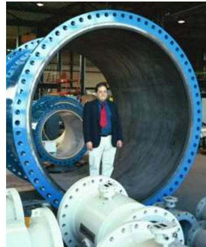
Dr. Yoder inside an 86-inch magnetic flowmeter
